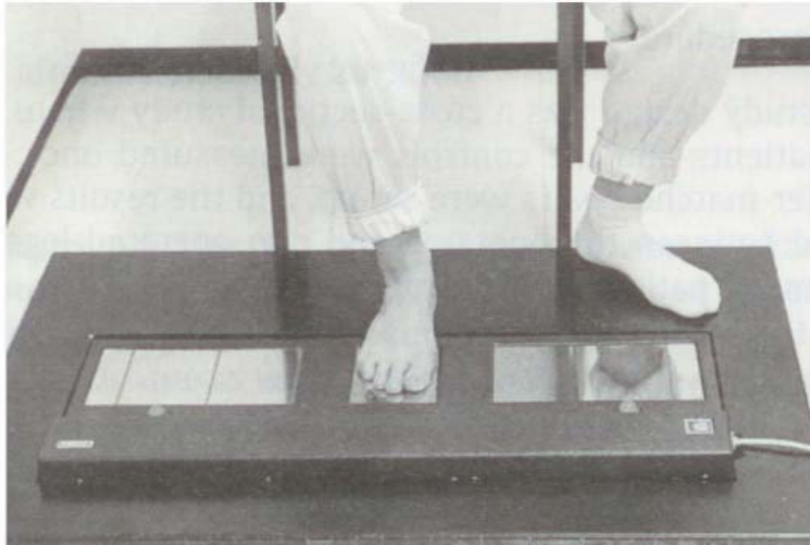
Fig. 7. The motor aspects of the feet were measured with the module for feet (BEP2) of the Human Performance Measurement/Basic Elements of Performance (HPM/BEP) system.
