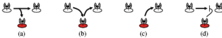
Figure 10. Different types of attacks in WSN: a) interruption b) modification c) fabrication d) interruption (Hamalainen et al., 2006).
