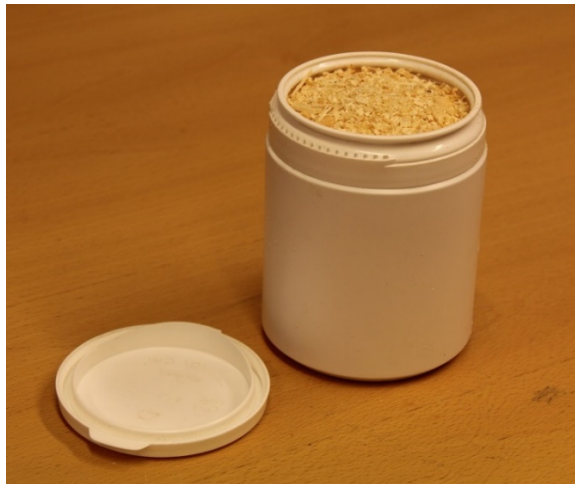
Figure 2: Valmet MR Moisture Analyzer. Left: NMR moisture measurement instrument; right: measurement container of the instrument with sawdust sample.
