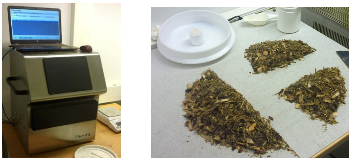
Figure 3. Left: Senfit BMA Desktop, the microwave moisture measurement instrument; Right: plate-shaped measurement bowl of the instrument with a crushed and milled stump sample divided into three parts.
