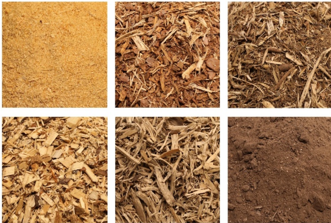
Figure 1. Solid biofuel samples from upper left corner: sawdust, non-fresh bark waste, non-fresh pruning residue, chipped small-sized trees, crushed and chipped stumps, and milled peat.
