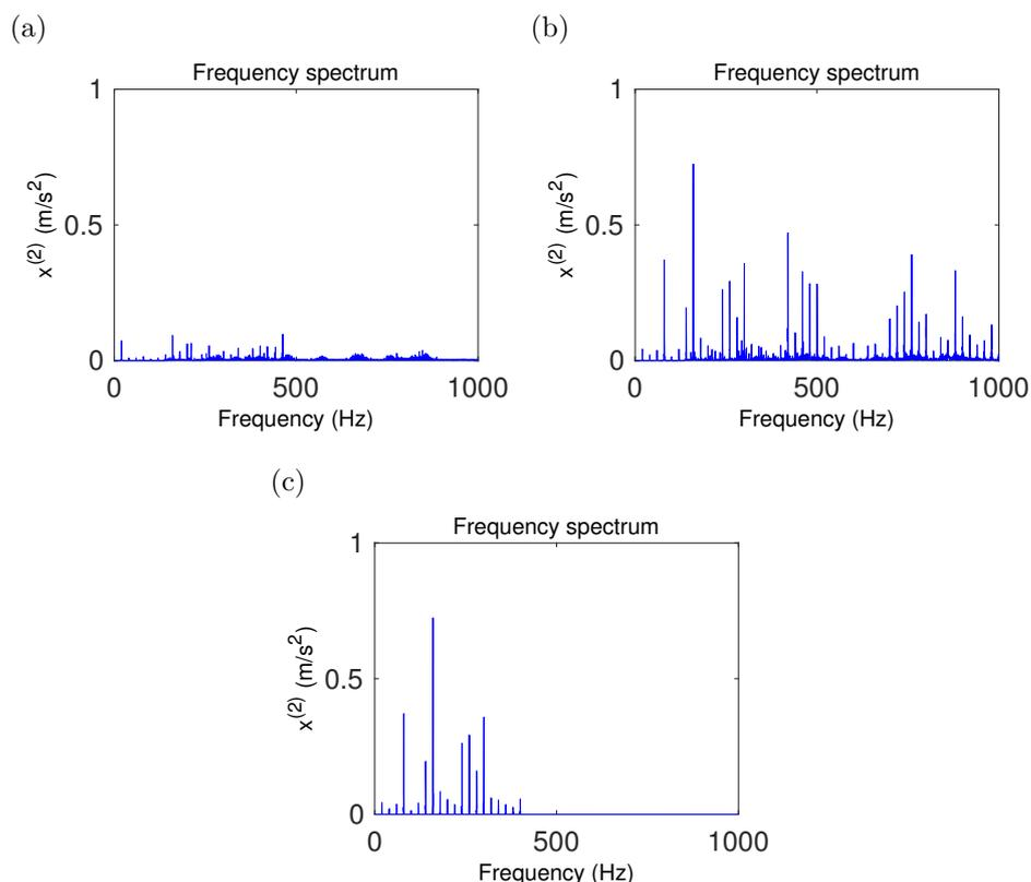
**Figure 6. Frequency spectra from three situations a) with no misalignment, b) with misalignment and c) with misalignment after frequency domain filtering**
