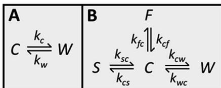
Fig. 4 (A) Two-site exchange model used to extract populations from chemical shifts and exchange rates from  $T_2$  relaxation times. C refers to the cage cavity and W to the window cavity. Kinetic constants representing the exchange of xenon from cage to window cavity and *vice versa* are  $k_C$  and  $k_W$ , respectively. (B) Four-site exchange model used in the analysis of the CEST spectra. S refers to the stuck window cavity and F to free gas.
