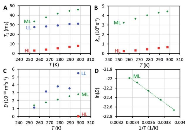
Fig. 3 (A)  $^{129}\text{Xe}$   $T_2$  relaxation times of xenon in CC3-R as a function of temperature. (B) Rates of xenon exchange between the window and cage cavities extracted from  $T_2$  data. (C) Diffusion coefficient of xenon in CC3-R as a function of temperature. The data of the LL sample is scattered because of the low signal-to-noise ratio in the experiment due to the low xenon concentration in the sample. (D) Arrhenius plot of the ML sample.
