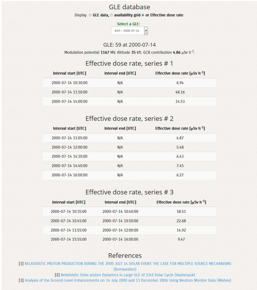
Fig. 1. Screen shot of the stored information about GLE 59 on 14 July 2000 in http://gle oulu fi/#/dose , namely the computed radiation doses at the cruise flight altitude of 35 kft (10668 m) for several different sets of derived spectra and the used bibliography. The numbering of the sets corresponds to the used references given on the bottom.
