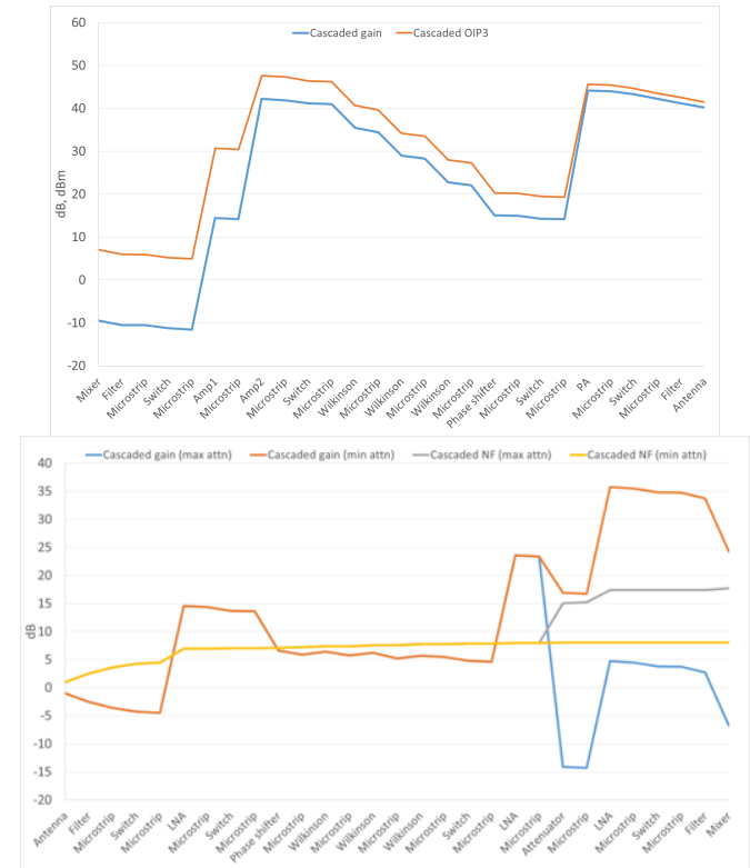
Figure 4. Cascade power analysis: (left) transmitter chain, (right) receiver chain.
