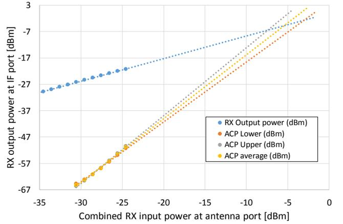
Fig. 8. Linearity measurement of array receiver to main beam direction.
