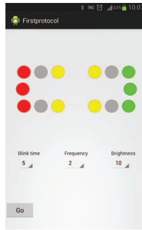
Fig. 5. The Android application sets indicator colors, frequency, brightness and blinking time and sends the visual cue to the device.
