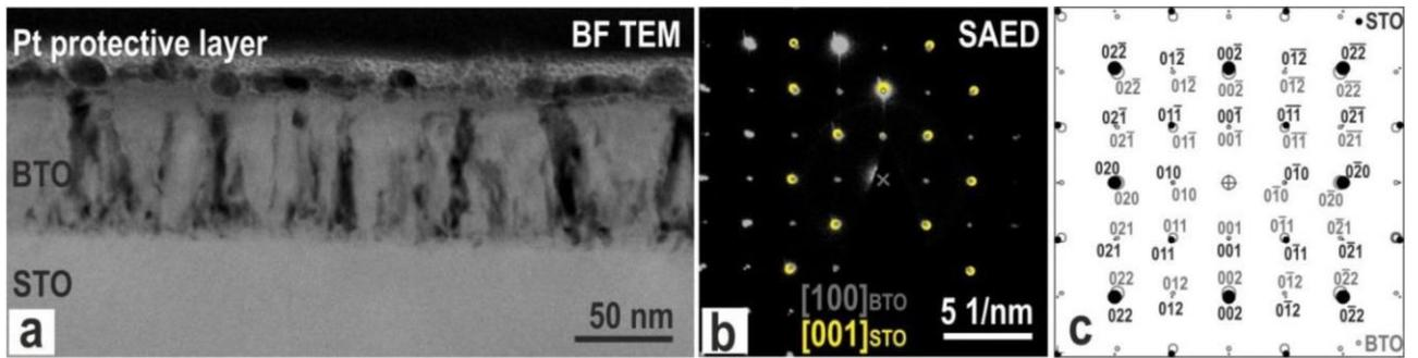
Fig. 4. TEM analysis of the BTO/STO cross-section. (a) BF TEM image. (b) SAED pattern in the [100] BTO direction. (c) Simulated diffraction patterns in the [001] STO and [100] BTO directions.
