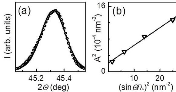
Fig. 3. (a) X-ray diffraction  $\Theta$ - $2\Theta$  scan around perovskite BTO (002) peak in the 70-nm-thick BTO film on STO. Solid curve shows the Gaussian fit. (b) The Williamson-Hall plot for the (00l) diffractions. Straight line shows the fit.
