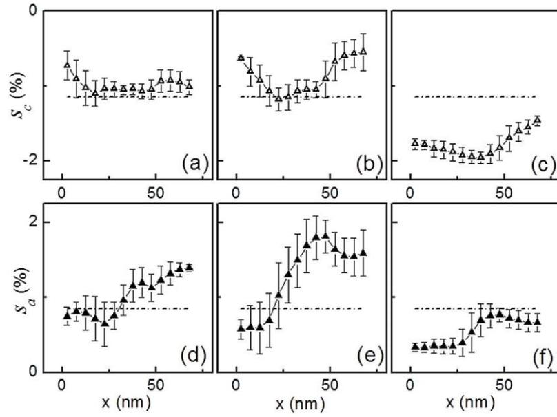
Fig. 6. (a–c) The out-of-plane strain  $s_c$  and (d–f) in-plane strain  $s_a$  determined by HRTEM/FFT analysis at three separate sites of the sample: site I (a,d), site II (b,e), and site III f). The average strains are shown by dashed lines.
