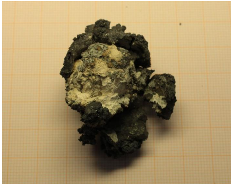
Fig.5 – Undissolved lime particle in the solidified slag sample. Sample is taken during the decarburisation stage.
