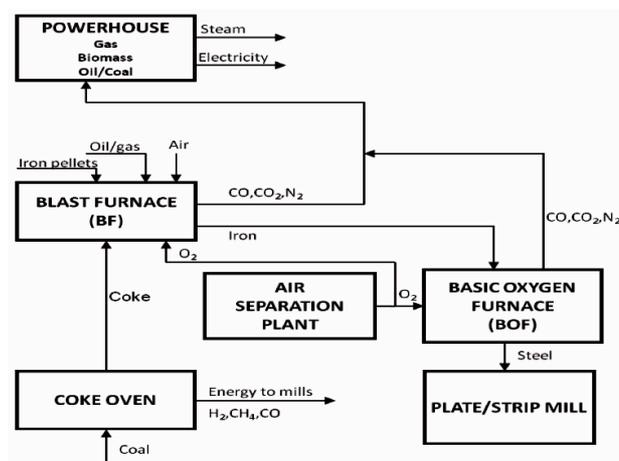
Figure 2. Typical production scheme of a steel mill.
