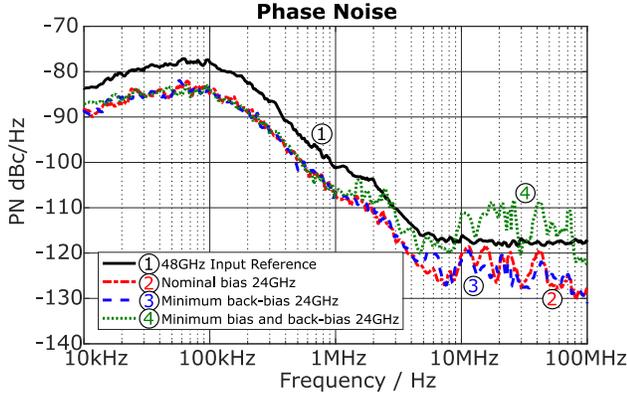
Fig. 4. Measured input reference and output phase noise.
