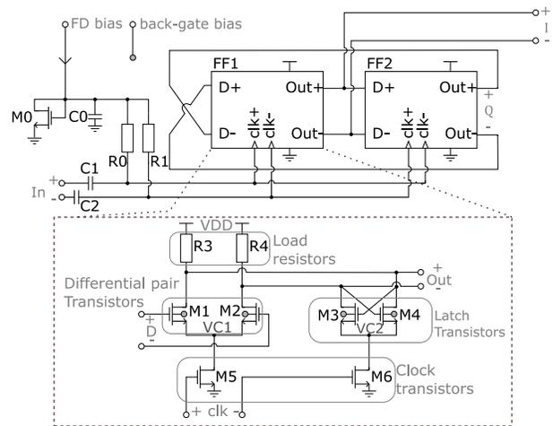
Fig. 1. CML frequency divider schematic. Input balun and output driver are excluded.
