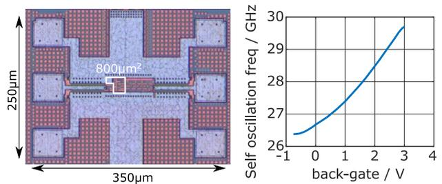
Fig. 2. Frequency divider chip micrograph and back-bias effect on  $f_{so}$ . Divider core is highlighted.
