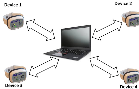
Figure 1. Wearable sensor system for multipoint measurements of blood perfusion
