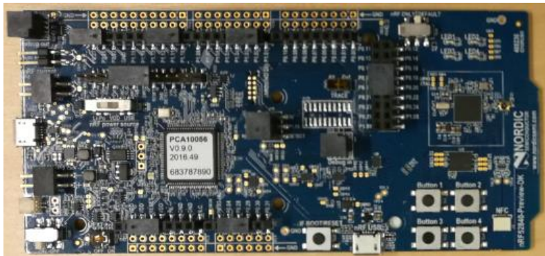
Figure 1. nRF52840 Preview DK device used for measurements.
