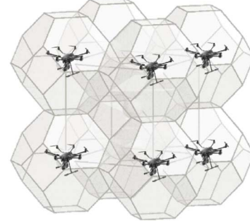
Fig. 3: Deployment of drone-BSs based on truncated octahedron cells.
