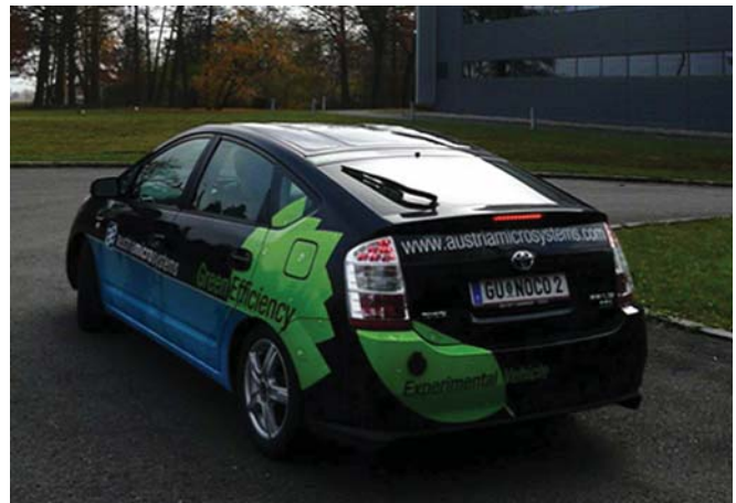
Fig. 1. Experimental vehicle with integrated PV cells on the roof
