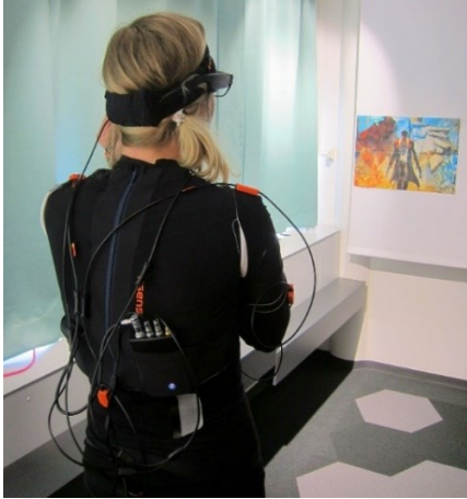
Figure 6. A test user with ODG R7 smart glasses and Xsens motion capture suit (ARMC).
