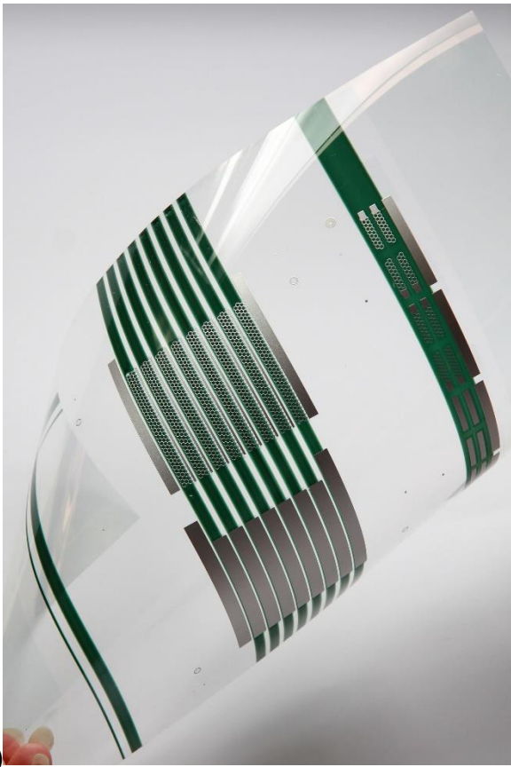
Figure 1 (a) Schematic representation of the OPV devices and (b) photograph of modules and cells in this study
