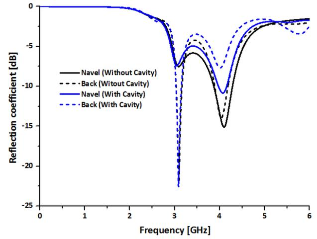
**Figure 12.** Simulated reflection coefficient of the UWB antenna with and without the cavity close to Navel and Back regions of the voxel model.
