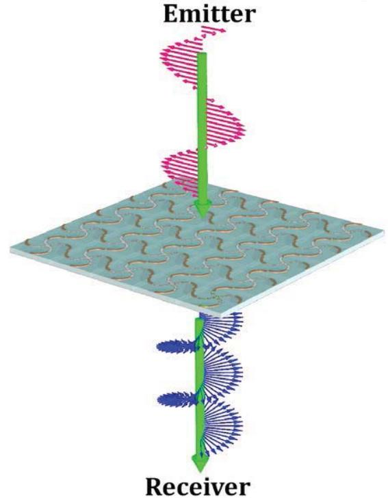
Fig. 2. The scheme of numerical simulation and polarization conversion.
