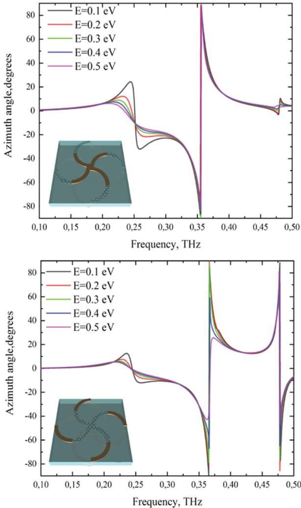
Fig. 3. Optical activity spectra for two types of the metasurface design
