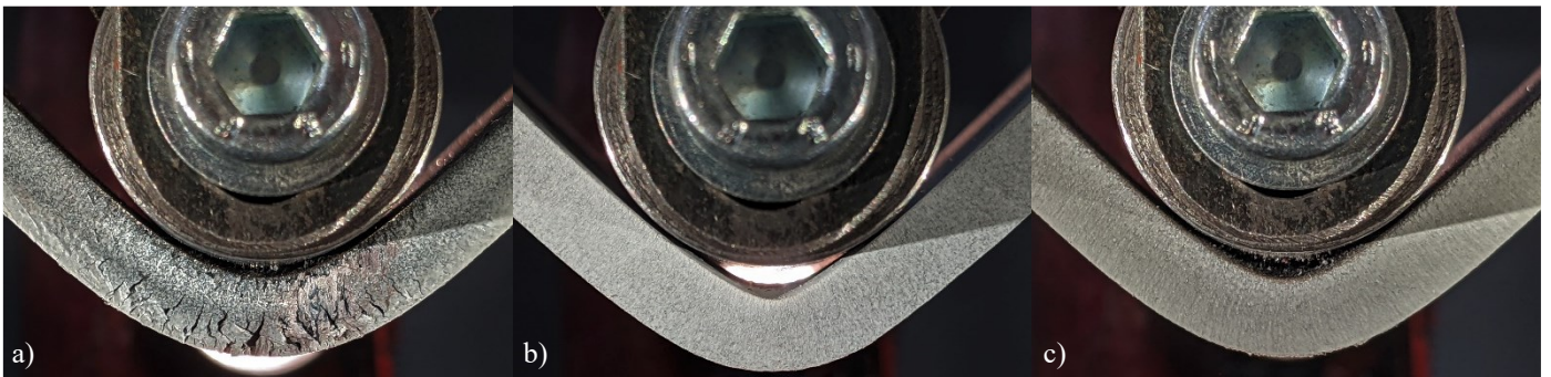
Fig. 2. Side-view images of (a) 700, (b) 900 and (c) 1100 MPa grades in the longitudinal direction (RD) at 90° bend angle.
