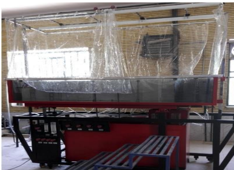
252 Fig. 3. Physical soil model and rainfall simulator used in laboratory tests.
