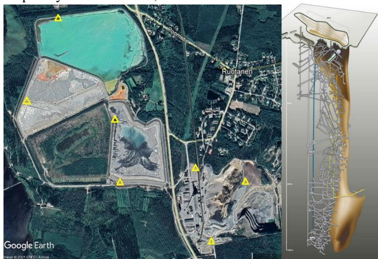
Figure 1. Pyhäsalmi mine area taken from Google Earth. Yellow triangles indicate the positions of corner reflectors designed for Copernicus earth observation satellites. The Callio Lab research activities utilise both the surface and the underground facilities of the 1.44 km deep base metal mine.
