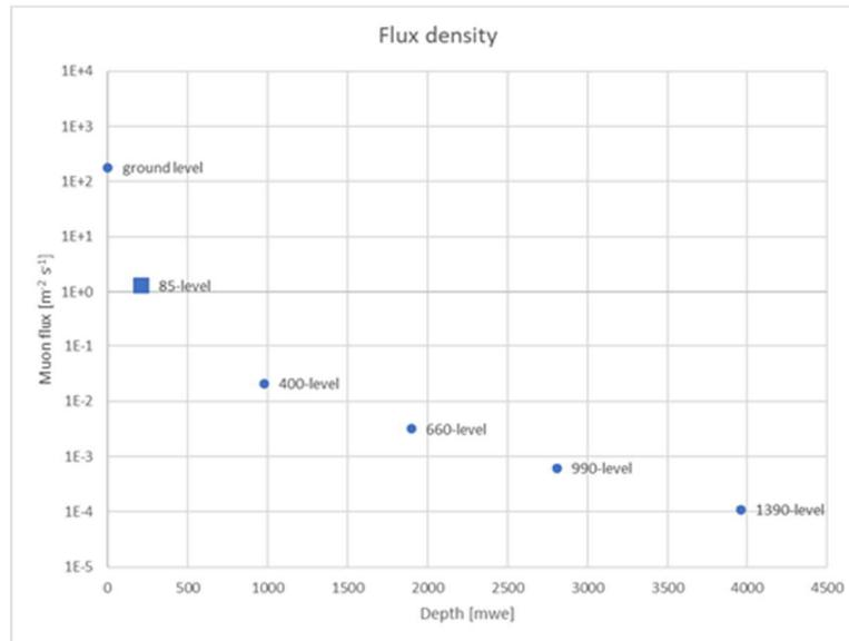
Figure 4. Measured muon flux at the Pyhäsalmi mine. Square marker is from the 2018 (14) EMMA measurement and round markers from 2005 measurements using the MUD instrument (15).
